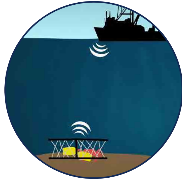
These pop-up systems remain on the seafloor until an acoustic signal is sent from an arriving fishing vessel.
