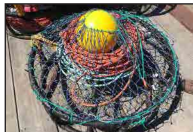
This Longsoaker gear uses the “timed release” method, where the line and buoys release at a specific time.
