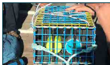
SMELTS gear also uses “on-demand release,” but with an inflatable bag instead of a line.
